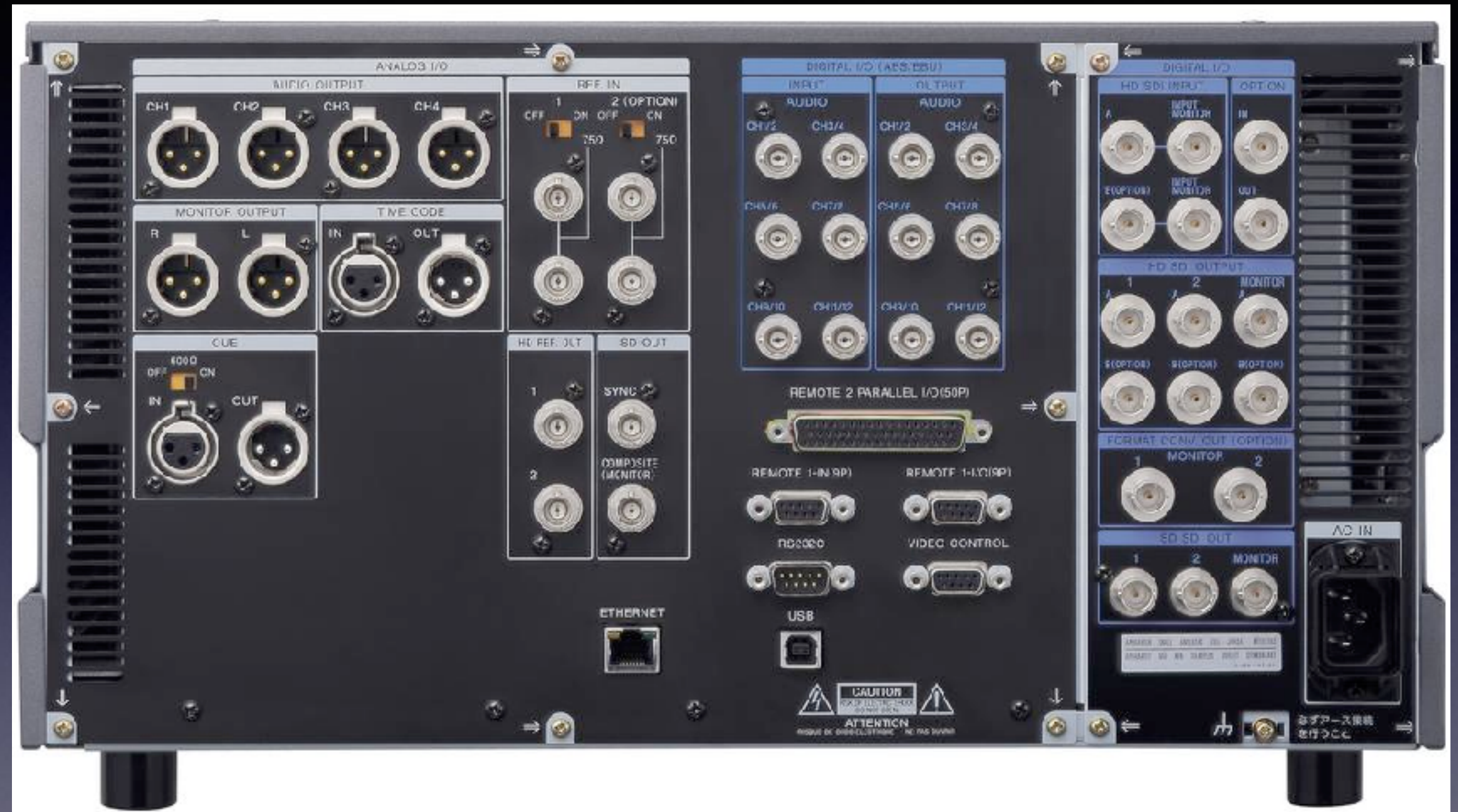
rear of srw-5500 HDCam SR deck
